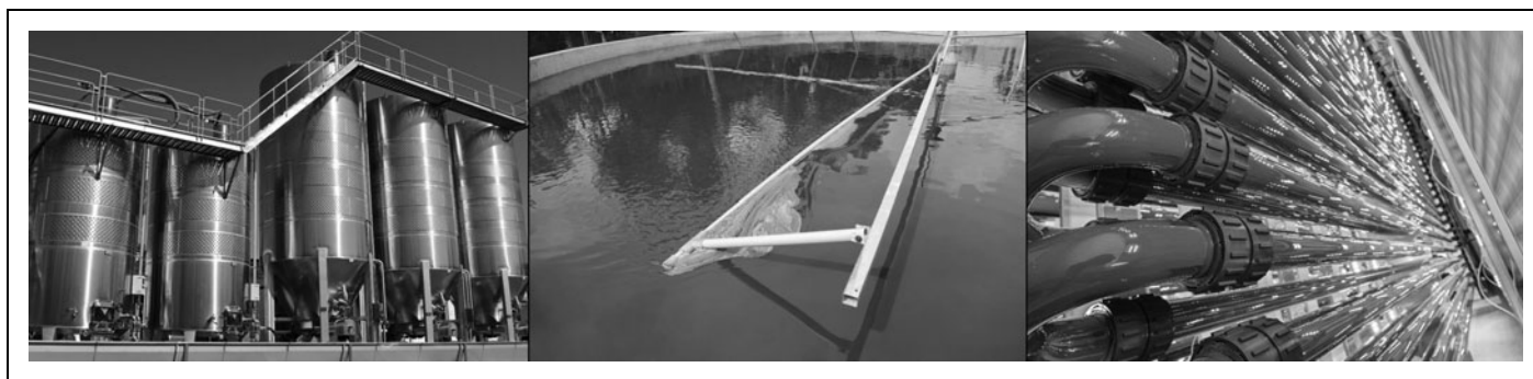
Fig. 2. Commercial algal cultivation systems: fermentation facility ( left ), open pond ( center ) and LED-based PBRs ( right , courtesy of Algalife).
